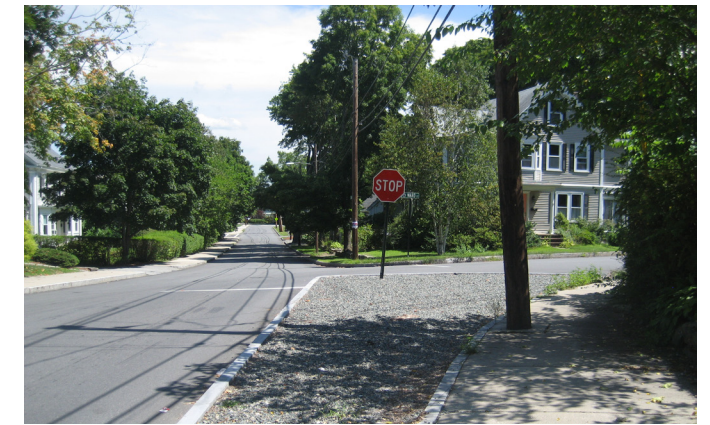
(A) Gravel-filled curb extension
